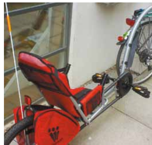
RIGHT: The seat can move to one of ten positions along the frame to set leg length, and the child's feet are secured to the pedals with Velcro straps. The chaining and chain are well guarded.
