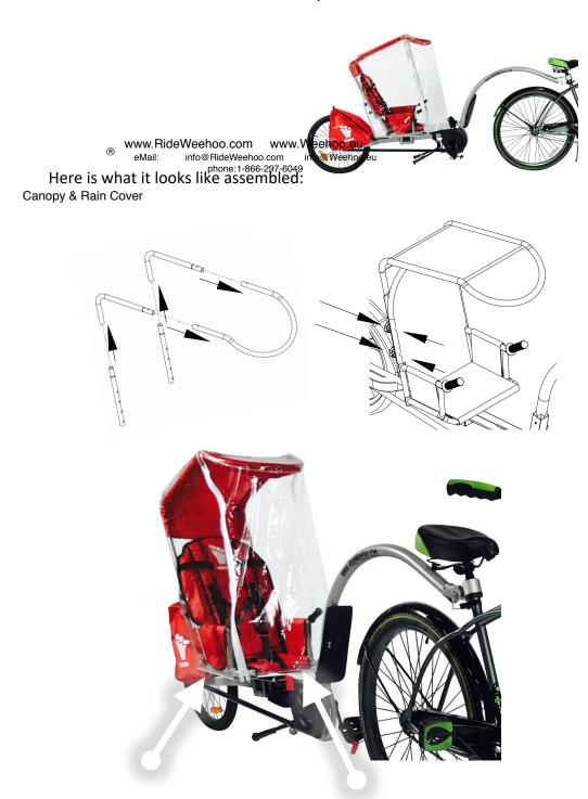
Insert white rods into the rain cover in the locations indicated: the two straight rods – one on each side, then the curved rod in the front. This keeps the rain cover rigid when riding.
